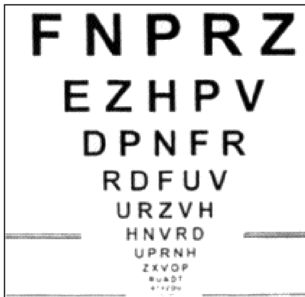
Fig. 3 SKILL CARD (High Luminance Side), Smith Ketterwell Institute, Low Luminance test card for evaluating near visual acuity, low contrast/low luminance vision and glare recovery in conjunction with a standard 5000 K photographic light box and stopwatch.
